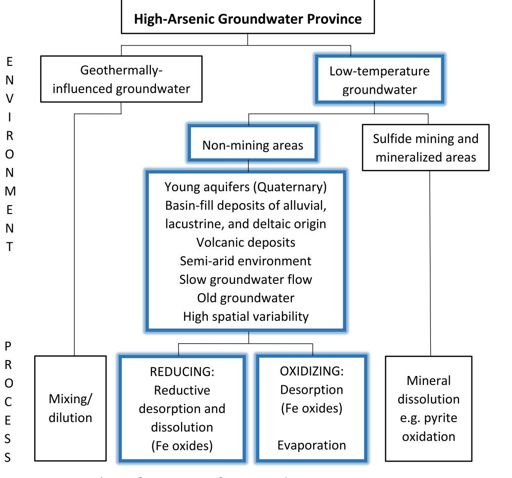
Fig. 1 – Classification of groundwater environments prone to As problems, highlighting local processes (modified from Smedley, 2001).
